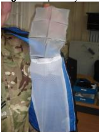
Fig 3. Cooling pack being fitted into the carrier
